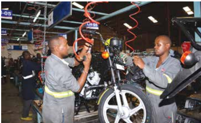
Assemblers at the Car and General plant in Nakuru put together TVS motorcycles using air tools. The moving line starts with a bare frame and ends with a complete ready for the road motorcycle every two and a half minutes. 200 bikes are produced each day to meet growing demand
